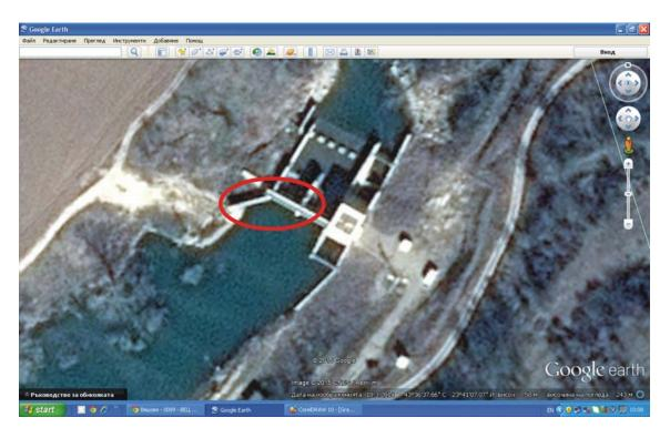
The next picture shows the barrage. Even if the steel barriers are uplifted at top position - the natural cross section of the river bed and its conductivity would still be reduced considerably.
